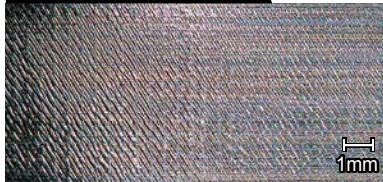
Worn / Cloudy surface
