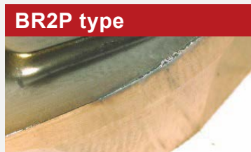
After six hours of cutting : Normal wear
