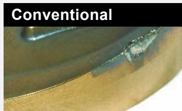
After an hour of cutting : Severely damaged; almost completely consumed
