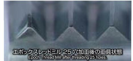
**タッピングが困難な超耐熱合金を加工可能!** It is possible to thread superalloy which is difficult to tap.
