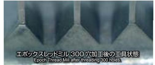
**300穴加工後も継続使用可能!** Machining up to 300 holes, NOT reached tool life.
