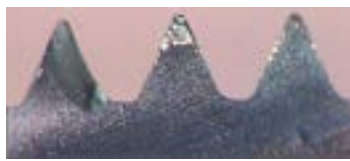
Conventional after threading 10 holes.
