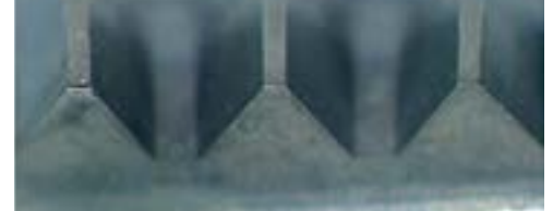
Epoch Thread Mill after threading 300 holes.
