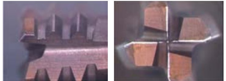
Epoch D Thread Mill after threading 600 holes.
