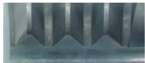
Epoch Thread Mill after threading 300 holes.
