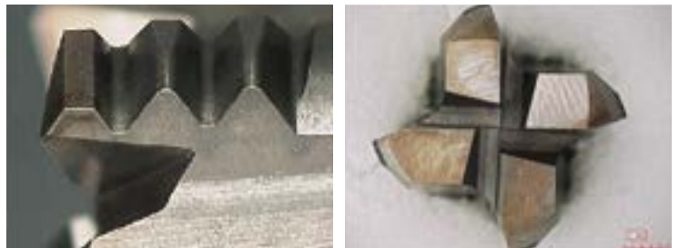
Epoch D Thread Mill after threading 64 holes.
