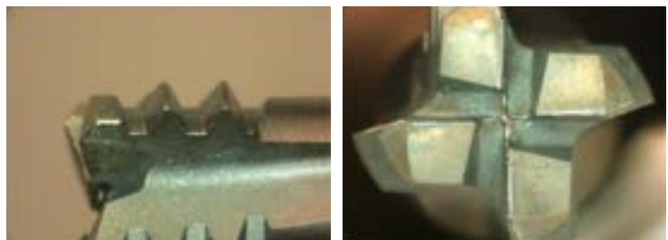
Epoch D Thread Mill after threading 150 holes.
