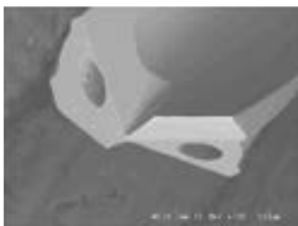
Tool wear after machining 1000 holes (25m)
